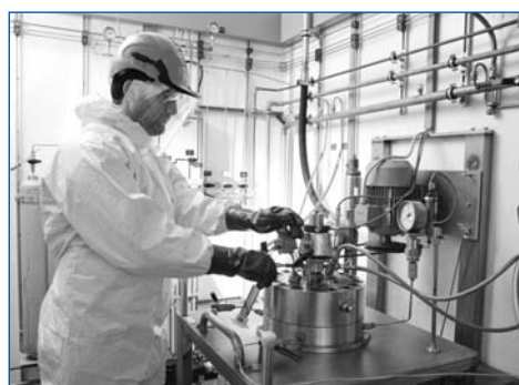
Figure 4. 16 Litre autoclave for reactions between -70°C up to 300°C and up to 300bar, safe handling of toxic and aggressive chemicals.
