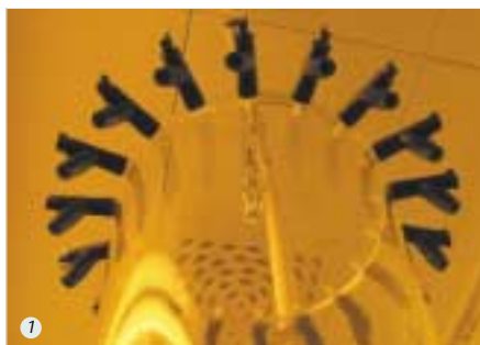
1 Lyophilizer in the amber light laboratory (for photosensitive compounds)
